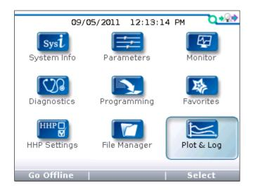
In the Main Menu, highlight the Plot & Log icon and press the "Select" softkey to go to the Plot & Log menu. You can return to the Main Menu at any time by pressing the Main Menu key ().
