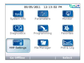
In the Main Menu, highlight the HHP Settings icon and press the "Select" softkey to go to the HHP Settings menu. You can return to the Main Menu at any time by pressing the Main Menu key ( ).
