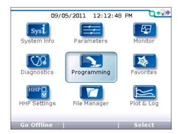
In the Main Menu, highlight the Programming icon and press the "Select" softkey to go to the Programming menu. You can return to the Main Menu at any time by pressing the Main Menu key ( ).
