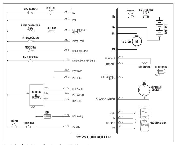
Fig. 3 Standard wiring configuration, Curtis 1212S controller.
