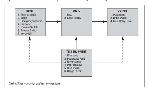
Fig. B-1 Safety channel block diagram, Curtis 1212S controller.
