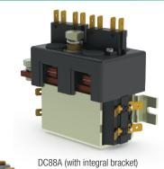
The DC88 motor reversing type of contactor has been designed for direct current loads, particularly motors as used on electric vehicles such as industrial trucks. The DC88 is a monoblock construction, resulting in a compact design which is compatible with modern electronic control systems. Developed for both interrupted and uninterrupted loads, the DC88 is suitable for switching Resistive, Capacitive and Inductive loads.
