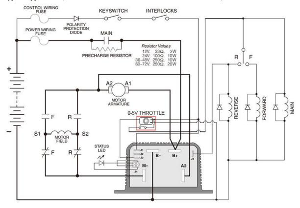
There are other wiring methods for connecting the IPPD throttle to a motor controller or 0-5V signal receiver (for example, an electric proportional valve). In same applications, the "Swith Out" (yellow wire, which is used as a security measure) may be left to be unconnected.
